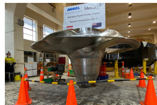
The final of the three new turbines ready for install inside the powerhouse in April 2025.
