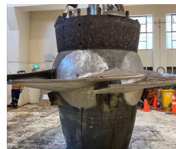
One of the original turbines removed from its chamber after decades of service.
