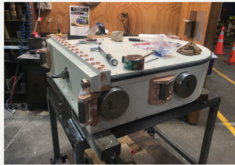
The priming valve of the gate being assembled in the AEC workshop.
